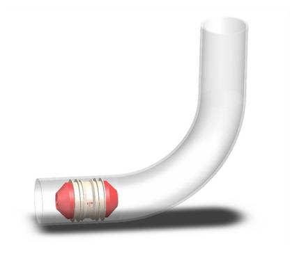
Residual liquids in the pipeline are difficult to remove. Pig with multiple lips inserted into the pipeline is pushed by air or nitrogen to thoroughly clean and remove any residues, leaving approximately 1 g/m in the pipeline. Pig speed can be adjusted by air pressure. Typical pigging air pressure is 3-5 barg.The system can be designed to remove static electricity.
